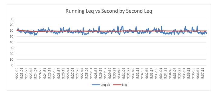
This chart shows the running Leq, the running average of the noise level in the sample, and the second-by-second Leq at NM1. Our goal is to ensure that the running Leq does not vary significantly for at least 5 minutes before the end of the measurement sample. This indicates that a larger sample would lead to a similar (and very likely nearly identical) noise level.
