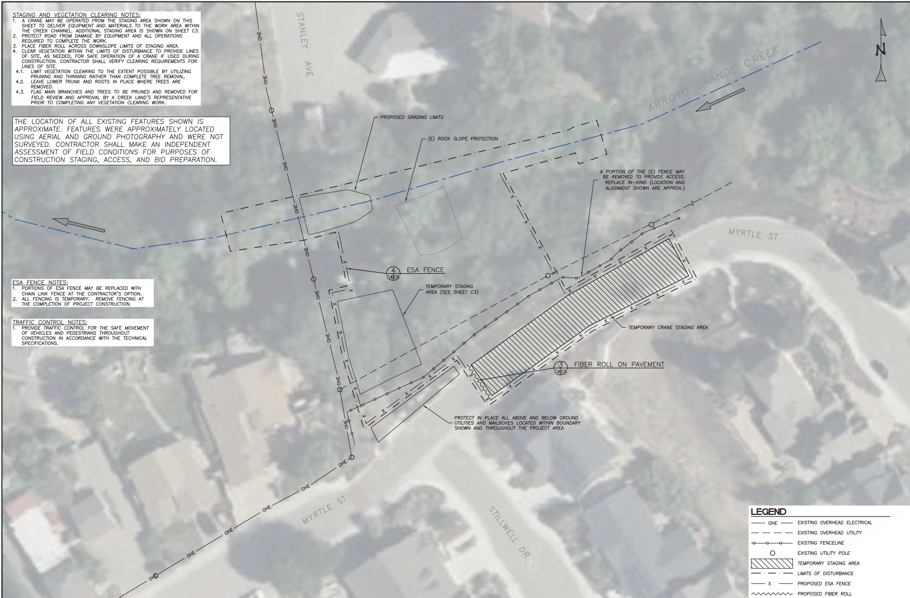
MYRTLE ST. CONSTRUCTION STAGING PLAN SCALE: 1" = 20'
