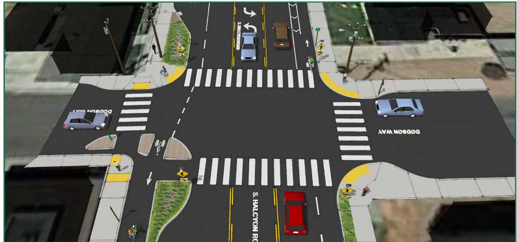
Buffered Bike Lanes and Curb Extensions at Halcyon Road and Dodson Way
