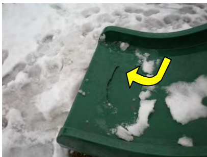
This tear could be an entanglement hazard.
