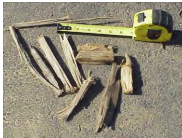
Exercise caution when purchasing recycled pallets for surfacing as large wood fragments can be hazardous.
