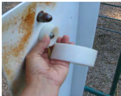
Gauges are used to test the compliance of all projections.
