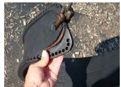
This strap swing is tearing.
