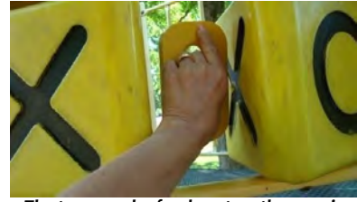
The torso probe freely enters the opening and therefore requires further testing.
