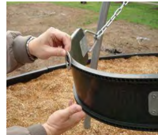
Test swings for protrusion hazards with this special gauge..
