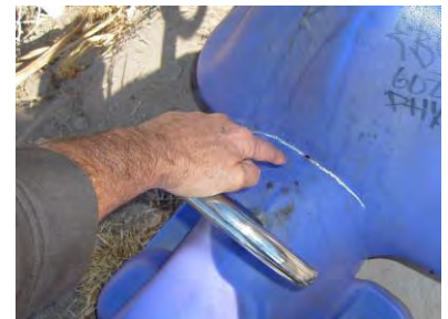
Cracked plastic could be a cut or scratch hazard.
