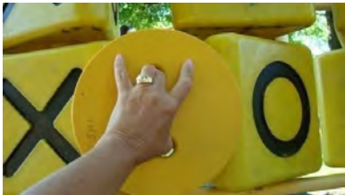
The head probe does not freely enter; therefore, this tic-tac-toe panel poses a head entrapment hazard and should be corrected.
