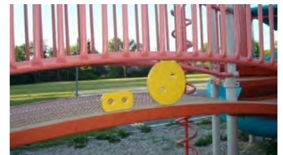
This photo shows the use of entrapment templates as opposed to the three dimensional probes.
