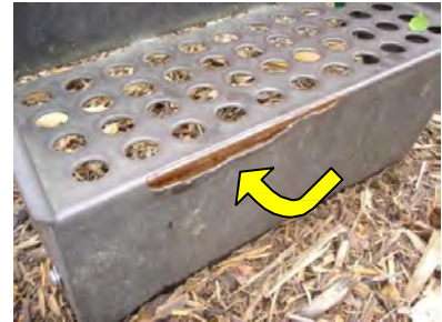
The PVC coating is peeling, exposing the metal underneath to the elements.
