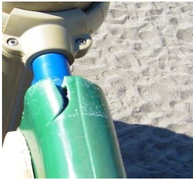
This cracked component is a hazard.
