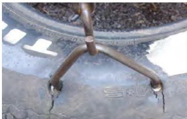
This tire is cracking.
