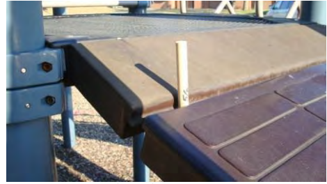
Demonstration of test for crush and shear hazard.
