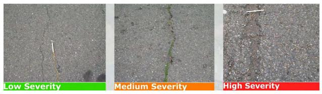
Image 4: Longitudinal and Transverse Cracking
