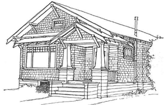
An extension of the early Bungalow, the Craftsman design included a low-pitched gabled roof with a wide, unenclosed eave overhang. Roof rafters are usually exposed and decorative beams or braces are commonly added under gables. Porches are either full or partial-width, with a roof often supported by tapered square columns. The most distinctive features of this style are the junctions where the roof joins the wall,
