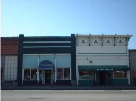
Characteristics included in late nineteenth century commercial architecture are double storefronts that are generally 25 to 50 feet wide with one or two entrances. Flat roofs and rooflines with detailed cornices, recessed entrances flanked by large display windows on the first floors and smaller vertical rectangular windows on the second floors are common as well. Materials of the time the historic commercial buildings in Arroyo Grande were built include stone, brick and wood.
