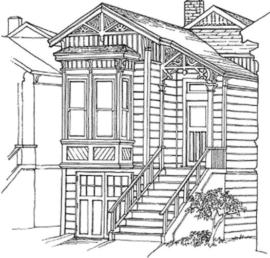
The Folk Victorian style uses a simple, folk type house style that is often one story and has a roof that is gabled or hipped (pyramidal). It lacks the intricate, irregular roof structure of the Queen Anne style, but includes ornamentation common to Victorian-style detailing, especially spindle work. Facades are generally symmetrical.
